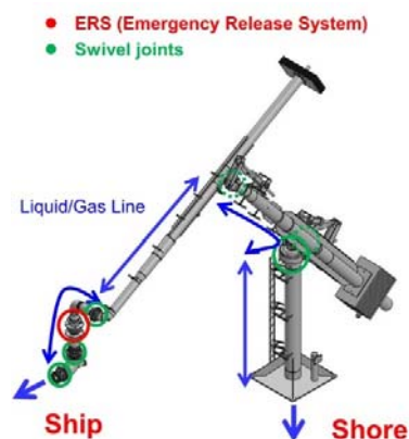
Loading arm for liquefied hydrogen under development at SIP
