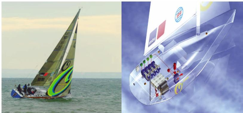
**MTU CFC presented this PEM fuel cell powered sailing boat in October 2003. The boat is powered by a 20kW unit, jointly developed with Ballard, which enables a range of 225km at a speed of 6km/h.**
