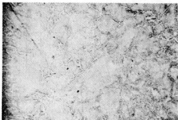
図1.3.5(a) B500試験片表層 ( $\times 100$ )
