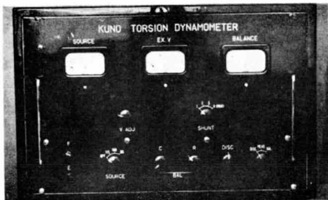
Fig. 3-15 Sources of electricity & amplifier of Kuno torsion-meter
