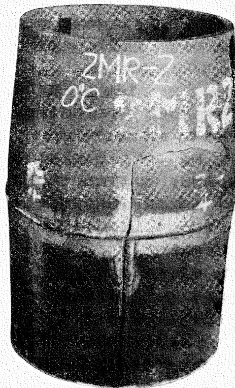
Fig. 2-22 An Example of Fractured Specimen of Explosion Test on Welded Pipe of Quenched and Tempered Steel. (800 mm in length, 400 mm in dia. and 20 mm in thickness). Showing that the Crack propagated along the Heat-Affected Zone of Welded Joint<sup>19)</sup>.
