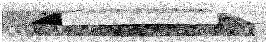
Fig. 3-25 Fracture at Heat Affected Zone of Heat Treated Steel
