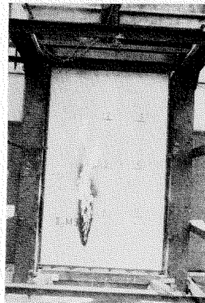
Photo. 28. IIБ M 9 Test Sample After the test, unexposed side wood started to burn.
