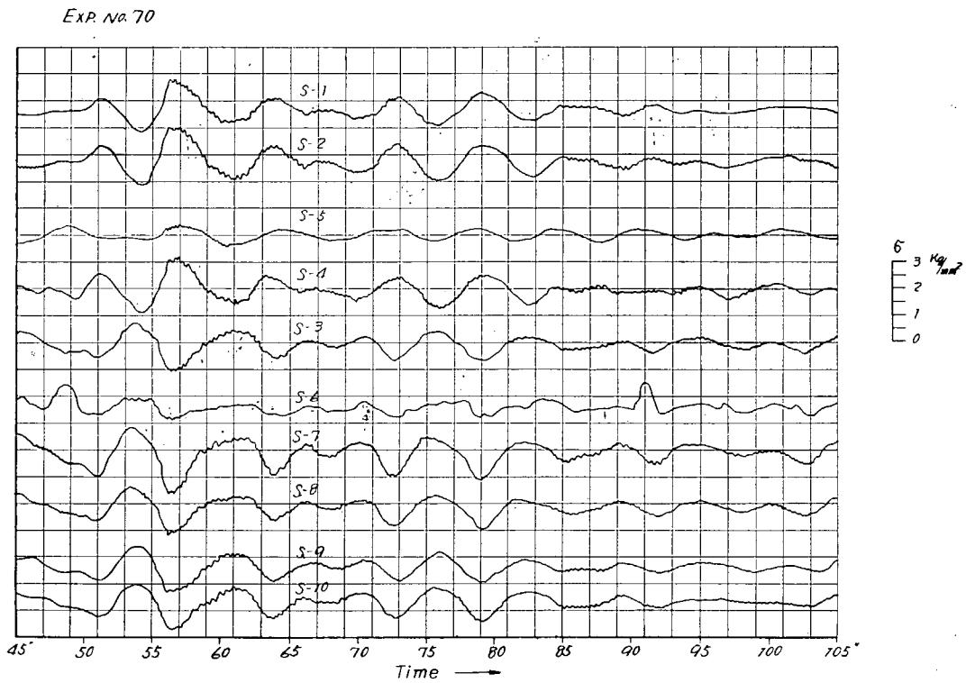
Fig. 5·5 Stresses in Midship Section
