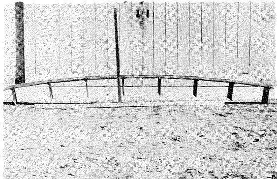
Photo. 5・3・3 Deformation in Free State
