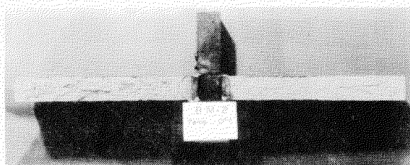
C-2. T=0^{\circ}\text{C} , \sigma_{n_1} = 25.1 \text{ kg/mm}^2
