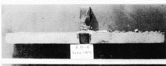
C-6. T=-78^{\circ}\text{C} , \sigma_{n_1} = 4.0 \text{ kg/mm}^2
