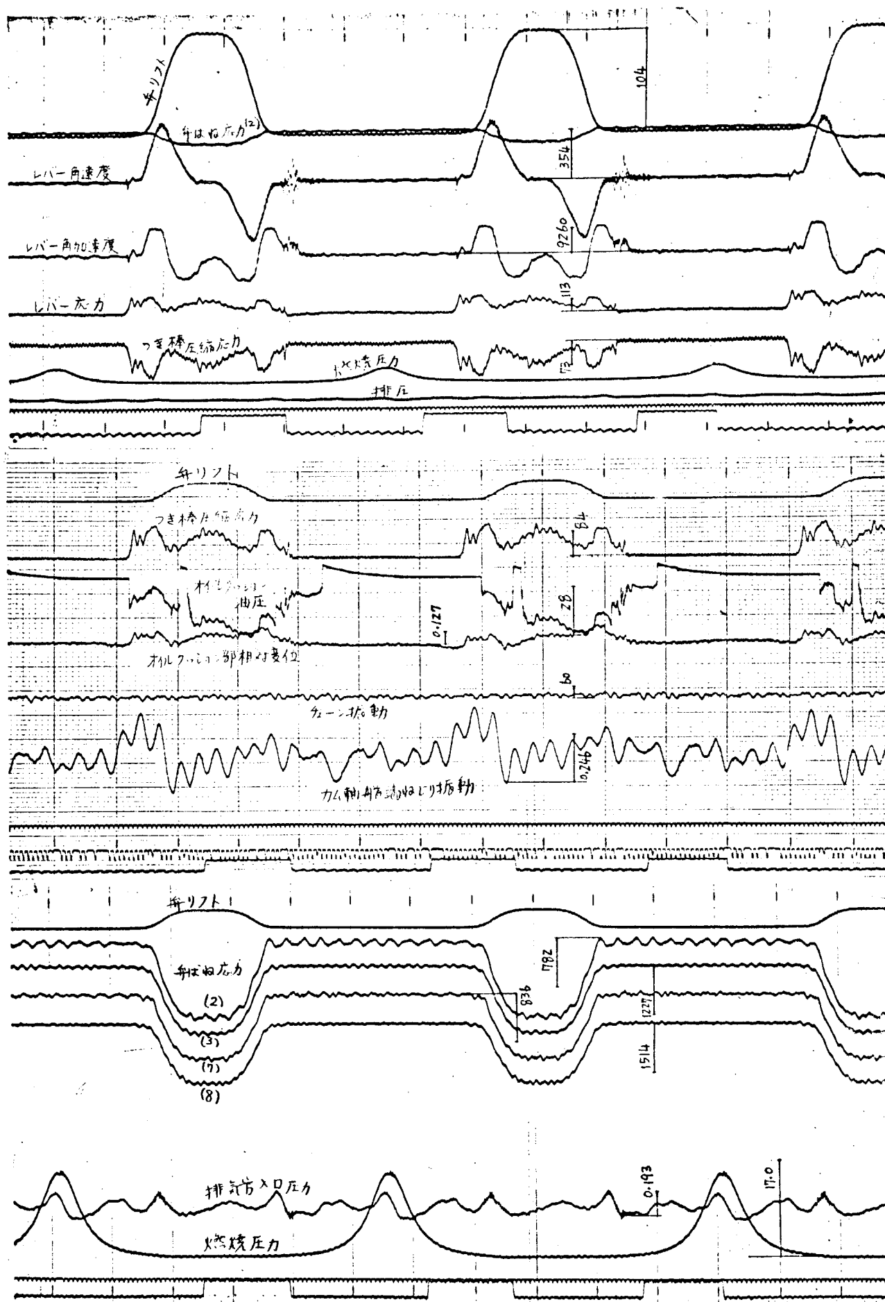
図8 運転時弁系振動 ( n_e = 110 \text{ rpm} , P_e = 0 \text{ Kg/cm}^2 , 計測3-4)
