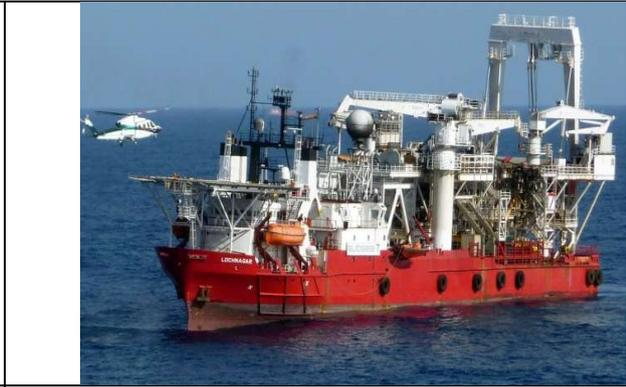
**PLSV - Pipe Laying Support Vessel**
