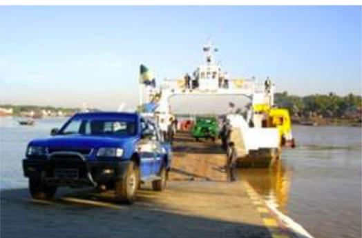
A Ro/Ro vessel unloading vehicles
