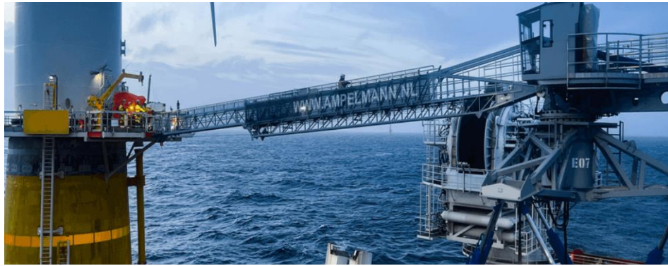
図 31 SOV with W2W Gangway Extended to Wind Turbine Tower
