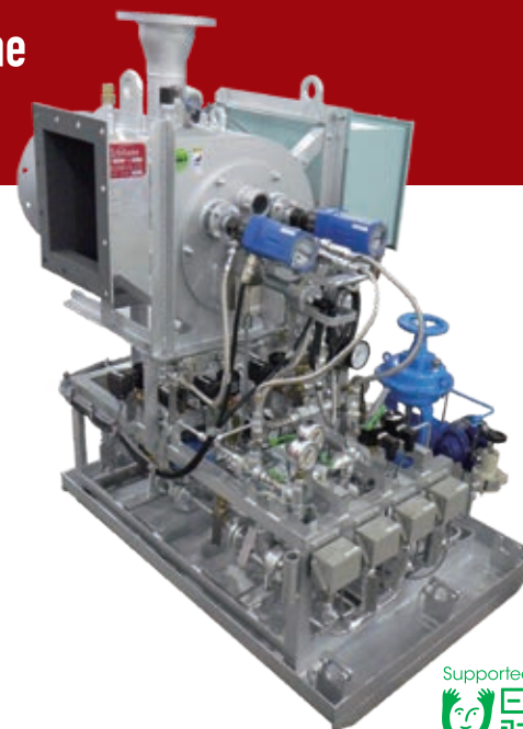
DF burner "Vignis" for auxiliary boilers
