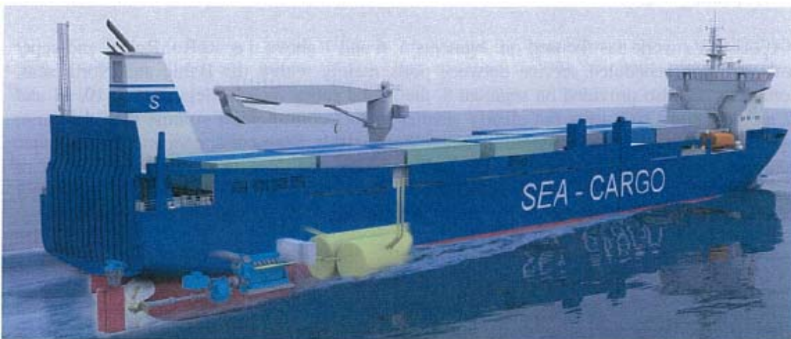
Figure 11: LNG-fuelled RoRo vessel ordered for North Sea trade. Illustration from Sea-Cargo AS
