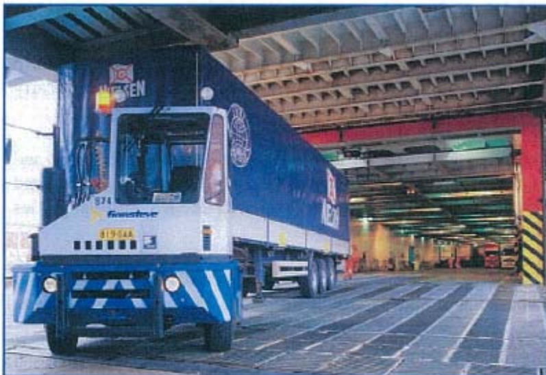
Figure 10: Loading a trailer onto a Ro-Ro vessel. Photo from Finnlines.
