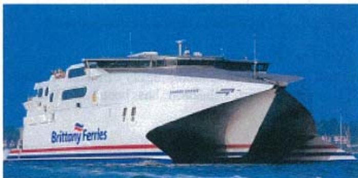
Figure 13: The "Normandy Vitesse", a 185-car fast ferry with 28,320 kW engine power and 41 knots service speed traversing the English Channel. Photo from Brittany Ferries.
