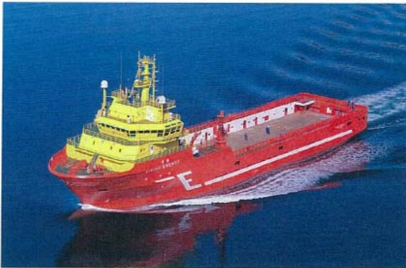
Figure 6: The "Viking Energy", and LNG powered offshore supply vessel operating in Norway since 2004 Photo from Eidesvik
