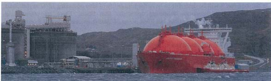
Figure 29: Large scale LNG: LNG carrier "Arctic Princess" (147,200 m 3 ) loading at the production facility at Hammerfest, Norway (4.1 million tonnes/year capacity). Photo: StatoilHydro
