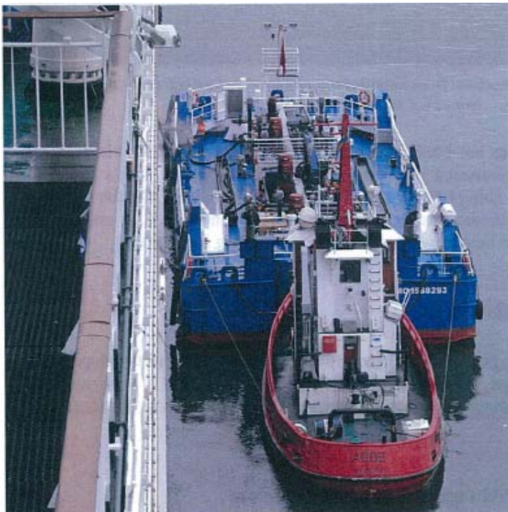
Figure 18: Bunkering barge for conventional bunker fuel assisted by tugboat.
