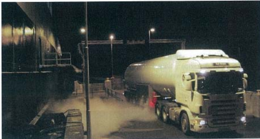
Figure 17: LNG bunkering at night from tanker truck at Arsvågen, Norway.
