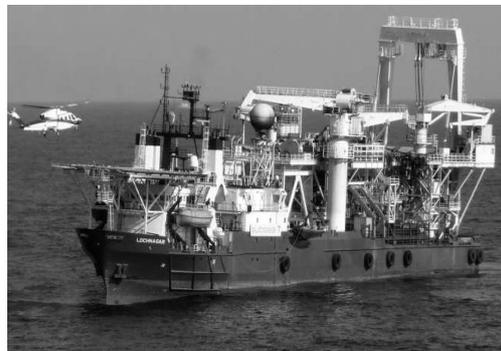
**PLSV - Pipe Laying Support Vessel
